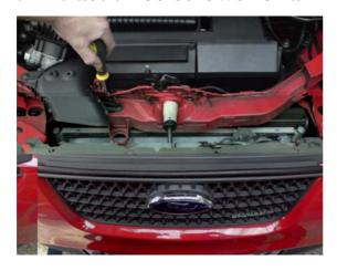
**3.** Remove ECU cover, this will slide upwards and then out.
