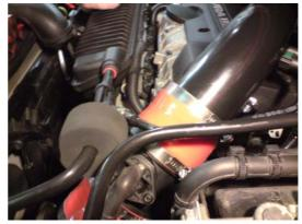
**26.** Now fit the filter and make sure that it is secure and it is not making contact with any other components.
