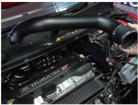
15. Check that all the bolts and brackets are present in the kit; fit the new DS Ind kit pipe into the turbo tube.
