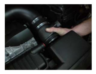
12. Slide the airbox out of the car to the right, be careful not to catch and damage anything when removing.
