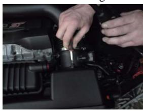
9. Remove air duct from the side of the air box.
