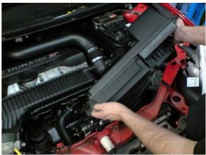
7. Remove electrical connection to MAF sensor.
