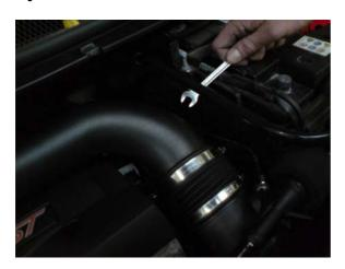
11. Pull MAF housing out of the standard airbox, remove seal from around MAF housing and keep in safe place as this will be needed if the standard airbox is to be re-fitted.
