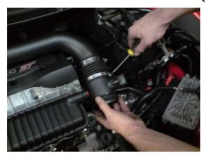
14. Remove the standard boost pipe by removing the 10mm bolt on the back of the pipe and the jubilee clip on the end of the pipe.
