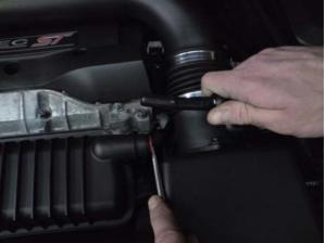
**10.** Remove 10mm securing bolt from the side of the cylinder head.
