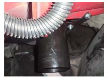
**24.** Attach the second pipe onto the maf housing then reconnect the vacuum pipe and MAF connector.
