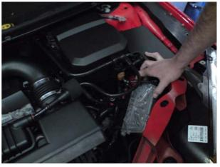
6. Remove Vacuum pipe from inlet manifold (push-pull fit)
