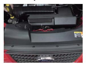
2. Extract three screws for air intake and remove.
